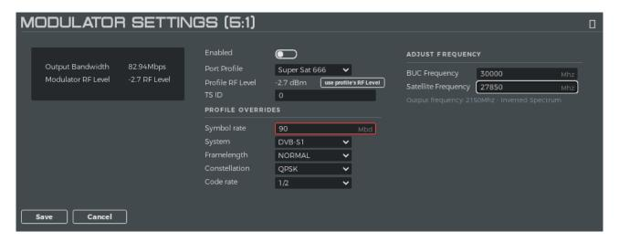
RF frequencies are given as Satellite Frequencies and BUC (Block Upconverter) Frequency. The resulting L-band Frequency out of the Modulator is shown as status.
