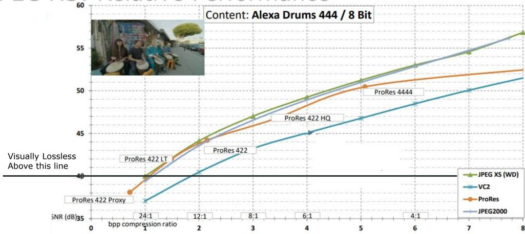
Note JPEG XS offers similar VQ to JPEG 2K at the same bitrate BUT JPEG XS does this with up to 5 times less hardware complexity AND with sub ms latency. XS is also specified to support the latest video resolutions, up to 8K, and streaming standards (ST2110).
