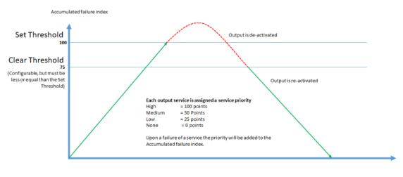
When a service fails, then it adds the priority points, when the total reaches the «Set Threshold» the outupt redundancy will take action.
