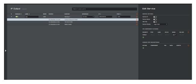
Mute on error will trigger when a service or services go missing from the MPTS with an aggregated priority of 100 or more. In the example above, the loss of just one high priority service will trigger MOE where as four or more low priority services would have to go missing to reach the threshold point of 100 and trigger redundancy protection. The threshold concept has been illustrated below;
