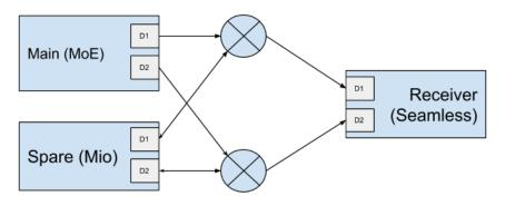
The diagram shows a main and backup chassis providing IP flows over a redundant distribution network. Let's say the intention is to use the chassis as a 1+1 redundant pair that delivers SMPTE 2022-7 coherent flows to a 2022-7 capable receiver. Adding the 2022-7 dimension highlights some of the behavioral aspects of the redundancy system which is the only reason this has been added.
