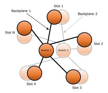
Management module 1 forms the core network of BP1 and management module 2 forms the core network of BP2 as shown in the diagram above.
