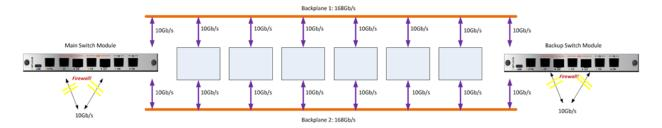
This network is provided in star form, with the switch/management module forming the central node of the network. All connections via the backplane to the modules operate at duplex speeds of up to 10Gb/s.
