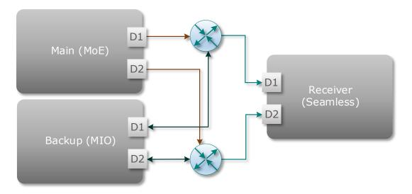
The backup chassis due to running exactly the same configuration as the main chassis will have all the output feeds muted. The Monitor-In-Out option will then monitor the output feeds from ports A and B from the main chassis and if a flow goes missing due to MoE or a network failure then the backup chassis will lift the mute for the required flow and output the content instead. When the main flow returns then the backup chassis will mute the output so that the main feed is active again.
