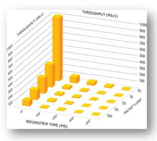
Using streaming techniques like HLS or RTMP did not work for PONANT. For a cruise ship near Australia, the roundtrip delay easily reaches more than 650ms. With the additional packet loss due to the VSAT's sensitivity to changes in weather, fog and ship movement, the bit rate plummeted to levels preventing broadcast-quality live video.
